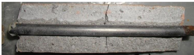
With RIS Chlore Fix Ace : No corrosion observed
